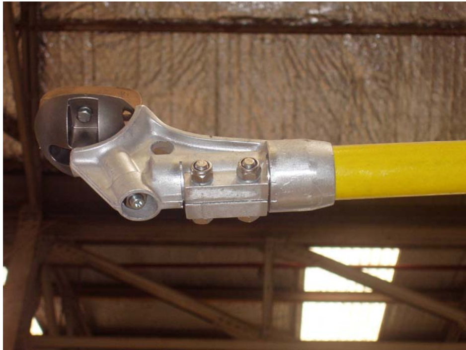
New Pole head fitted to fibre glass pole
