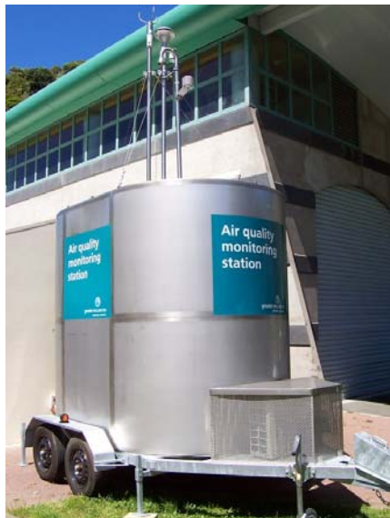
The mobile traffic emission monitoring station @ Ngauranga Gorge
