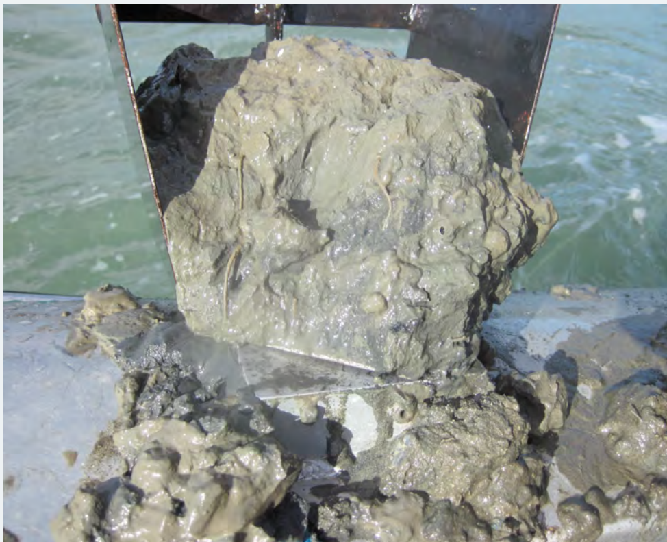
Sediment sample from the central basin of the Onepoto Arm - Jan. 2014 showing soft oxygenated surface muds (3-5cm light brown layer) overlying deeper more enriched and oxygen depleted (grey) muds. Note that the very soft and unconsolidated mud samples generally lost cohesion and collapsed after being removed from the water.
