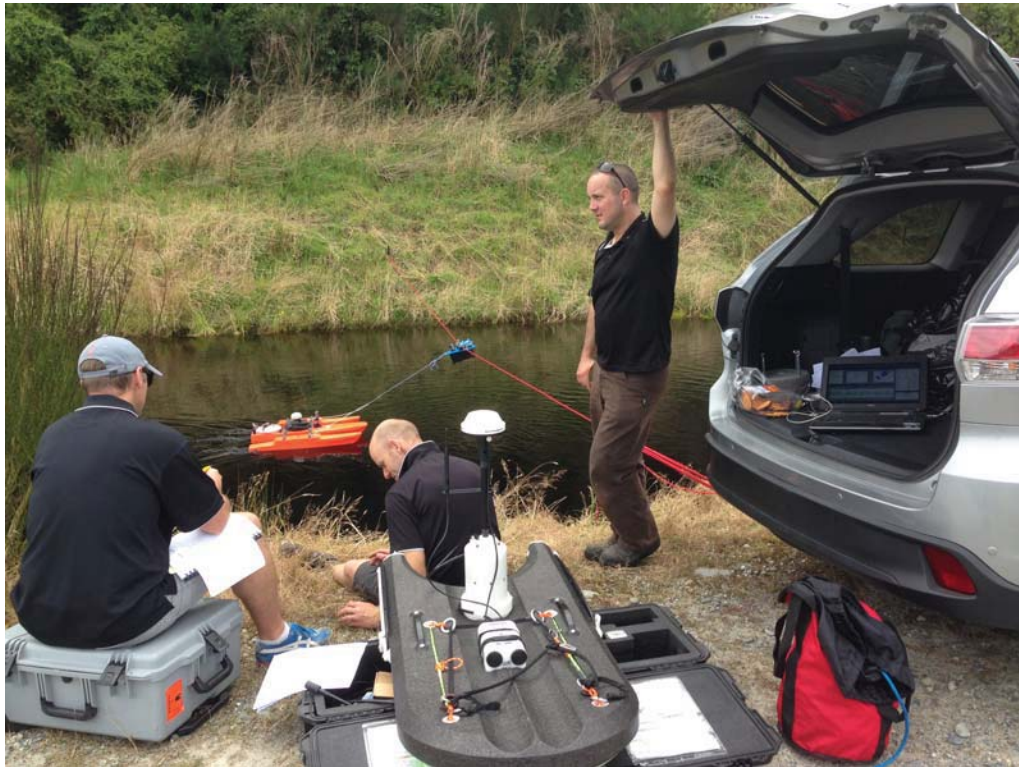
ESci staff using an ADCP to gauge the Dilmanstown Canal (Kumara)
