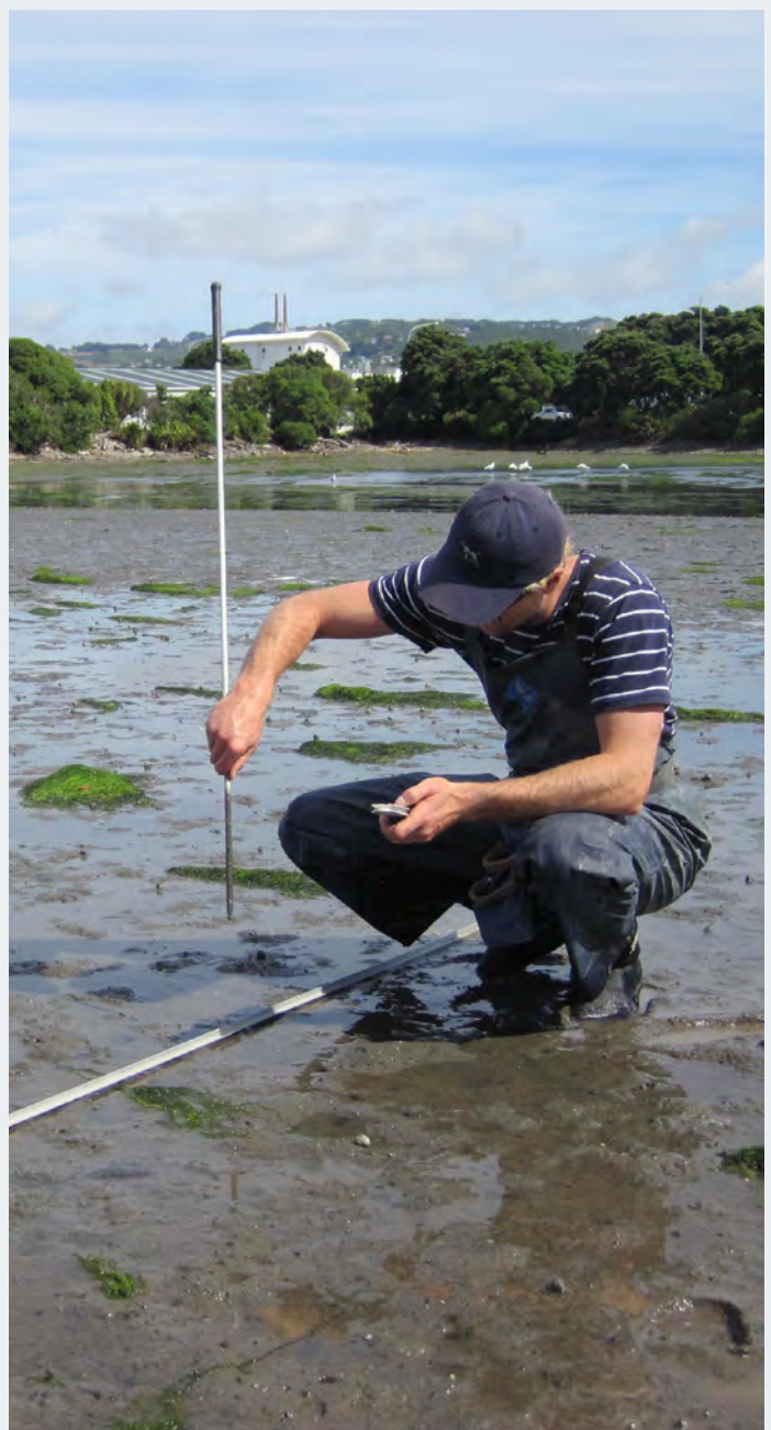
Measuring sediment plates in the lower Hutt Estuary, Jan 2016.
