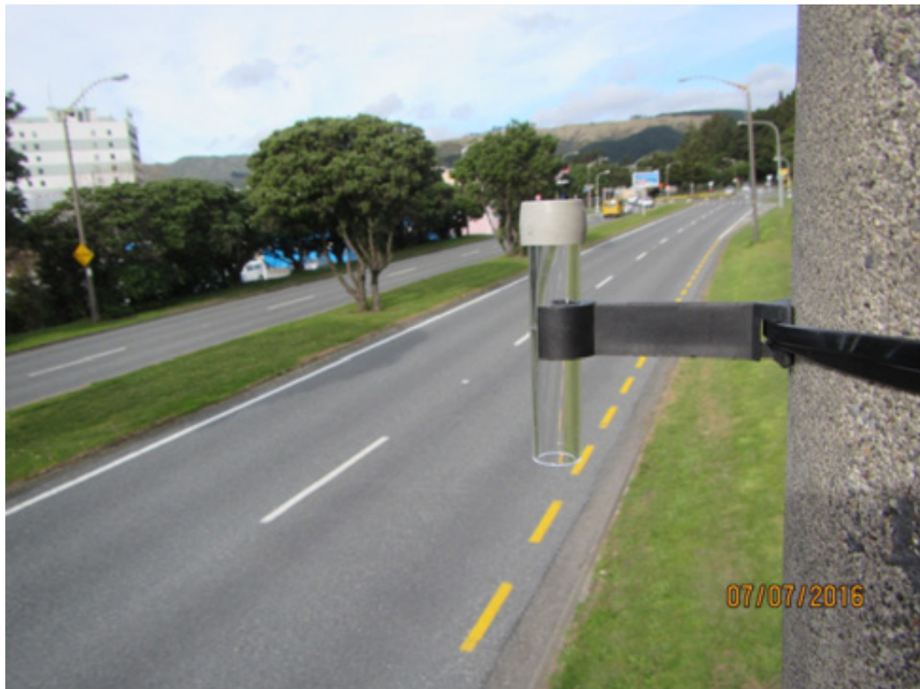
Figure 4.1: Passive diffusion tube mounted on street pole adjacent to Titahi Bay Road, Porirua (WEL080)
