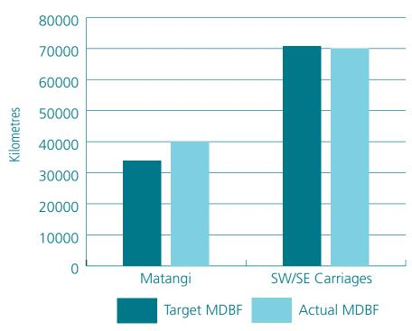
Fleet reliability for the year met the increased targets required in the partnering contract, a lot of time and resource has been devoted to ensuring that the reliability of the fleet is correctly measured and reported. This information can then be used to try and improve performance going forward.
