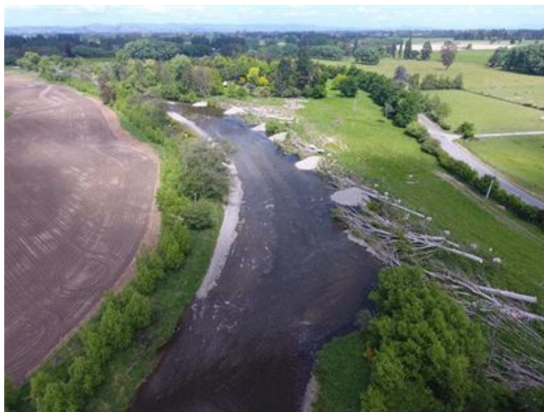
Photo 3: Waipoua River: Poplar tree removal, willow & native tree planting & gravel groynes near Matahiwi Rd
