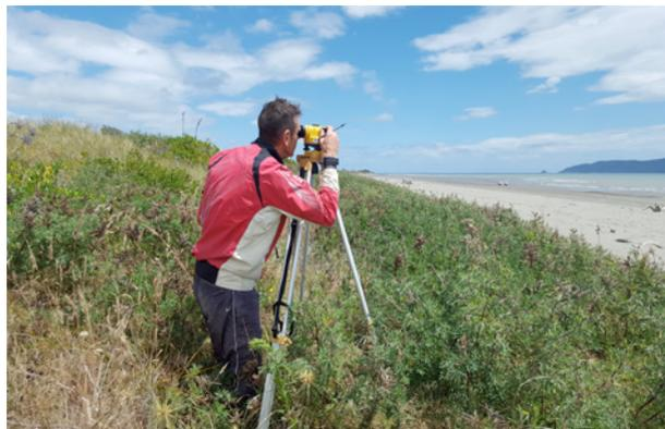
Cross-shore profiles from the top of the dunes to the shallow subtidal were measured using a theodolite.
