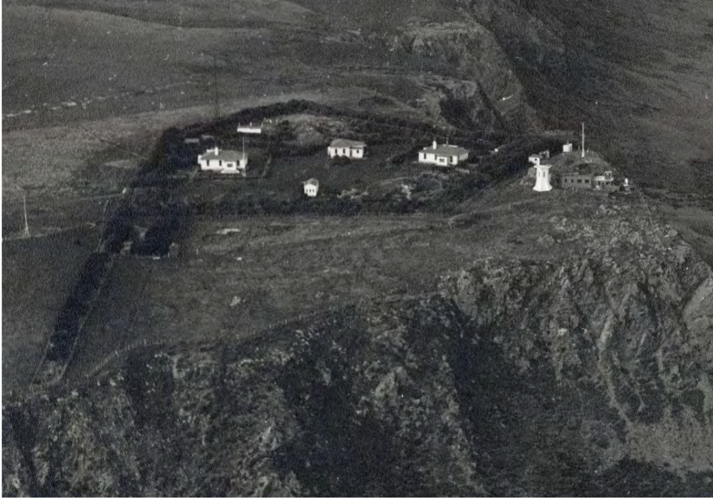
Fig. 3. Detail of Whites Aviation aerial oblique from the west. The date is estimated to be in the 1950s. Some salient features deserve note: 1) radar hut with possible aerial and barracks by the light, 2) signal mast, 3) signal hut (left of the mast)? 4) both no. 1 and no. 2 houses have small third bedrooms off the entry hall, 5) the second (WAAC?) barracks has been demolished. Courtesy National Library/National Archives ABPL W5221.
