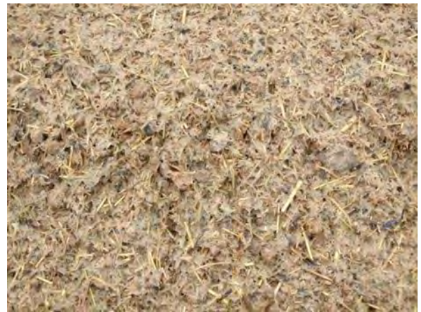
Figure 56: Hydrohay as applied
