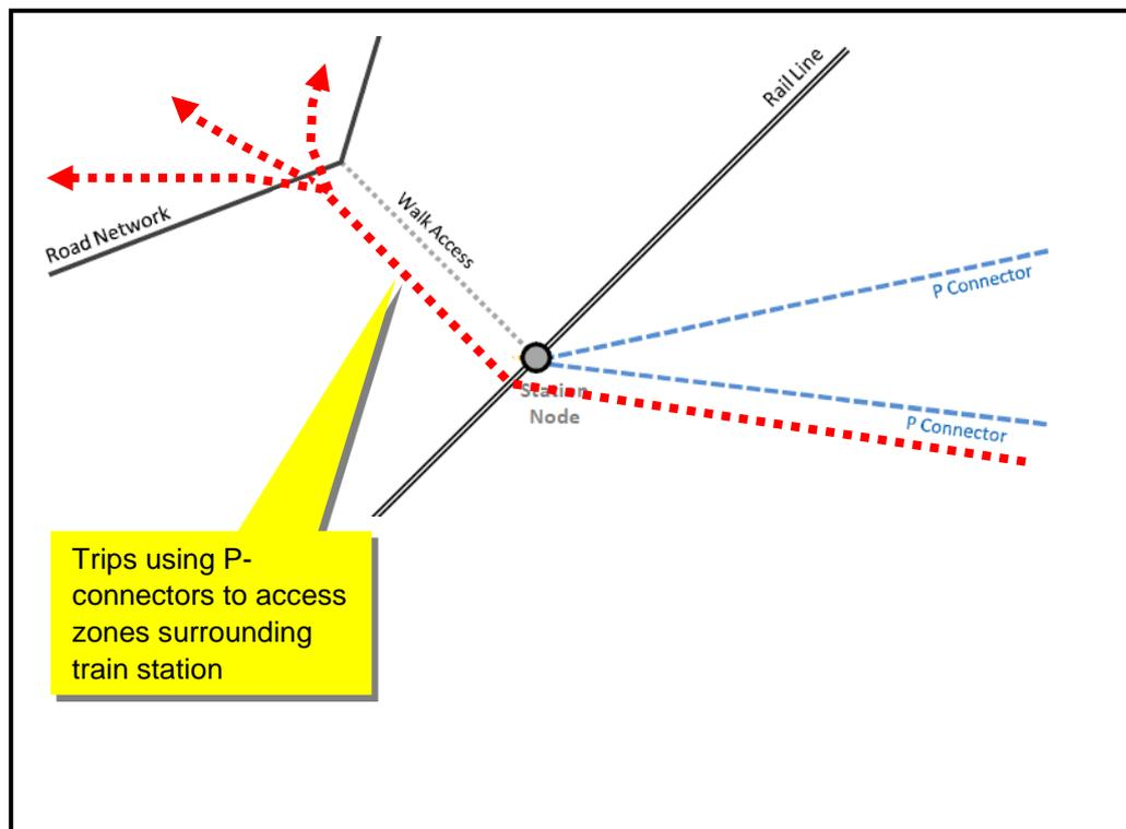
Figure 2-7: P-Connector Arrangement in the 2001 Model
