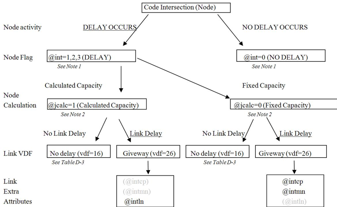
**Figure 2-10: Intersection Coding Flow Chart**
