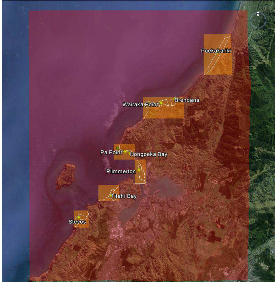
Figure A6. Levels 3 (red) and 4 (yellow) model nest grid extents for the West Coast - South (wsts) area
