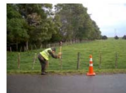
Seismic shot (sledge hammer) in action. Typically 3 shots (stacked) at each location.
