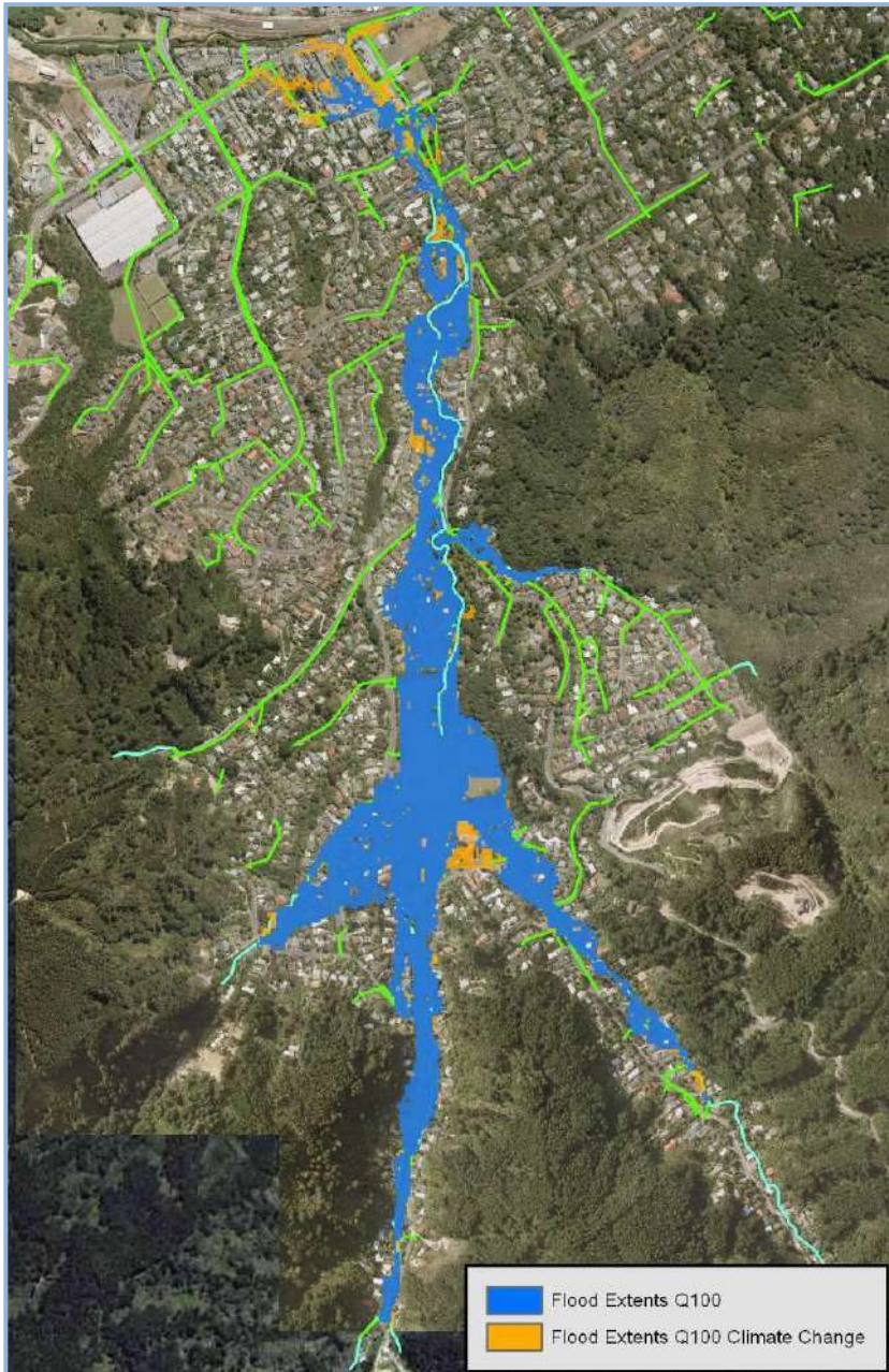
■ Figure 18 Comparison of Flooding Extents for Q_{100} vs. Q_{100} including Climate Change
