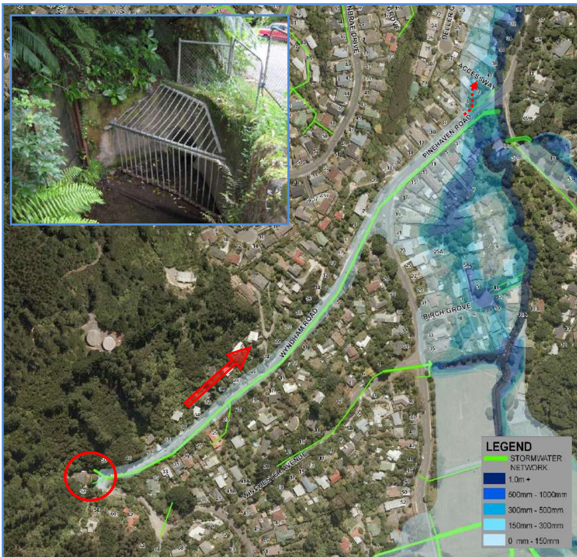
■ Figure 27 Predicted Wyndham Road secondary flowpath should inlet blockage occur during a 100 year storm
