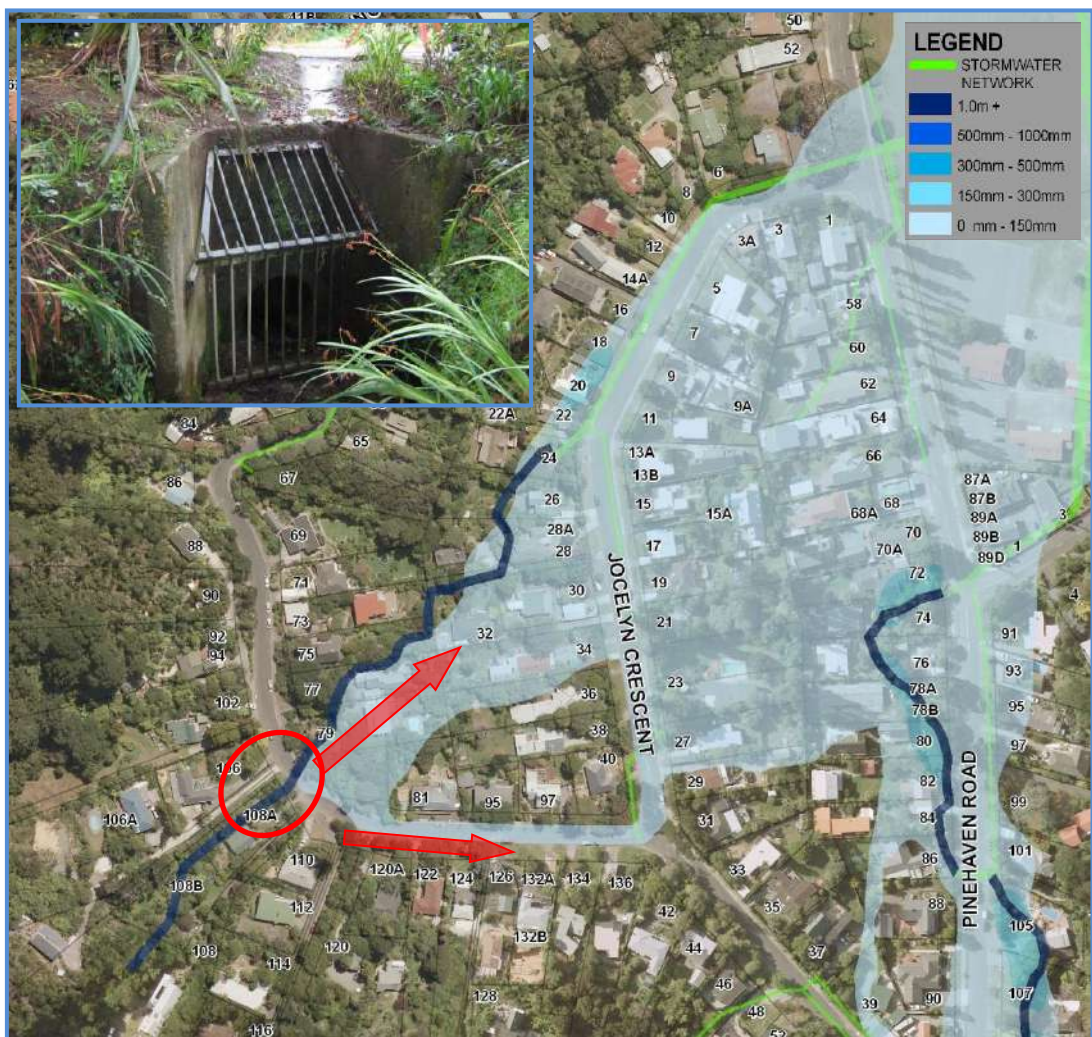
■ Figure 26 Predicted flood extents in the vicinity of the culvert under Wyndham Road in a 10 year storm
