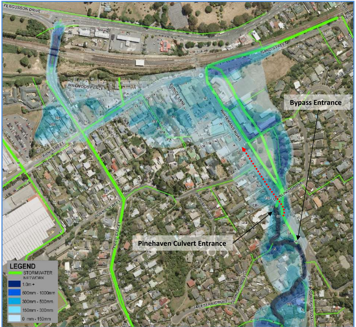
■ Figure 36 Predicted flood hazard extent in the lower Pinehaven Catchment during a 100 year storm event and a 50% blockage of the bypass and the piped section of the Pinehaven stream
