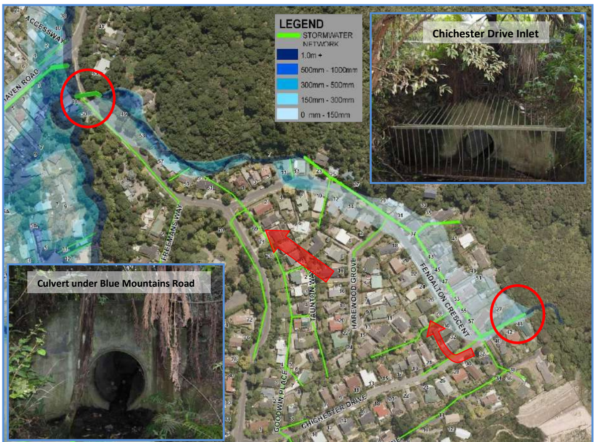
■ Figure 28 Predicted flood extents in Fendalton Crescent and Chichester Drive during a 100 year flood event and a blockage of the inlet of the Chichester Drive
