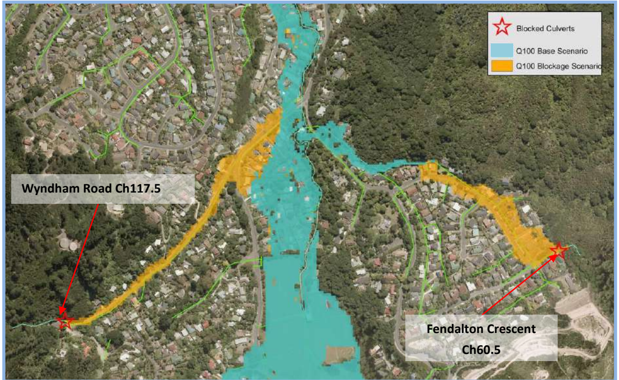
■ Figure 17 Comparison of Flooding Extents for Q 100 With and Without Blocked Culverts
