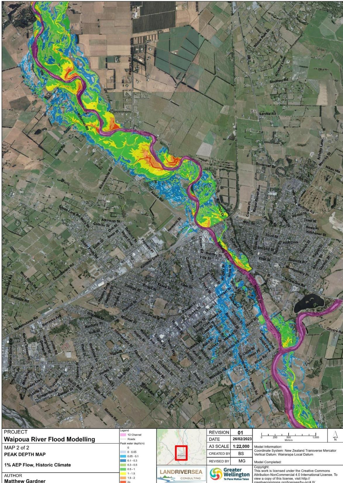
Figure 3.2: 1% AEP flood depth, historic climate, no sensitivity
