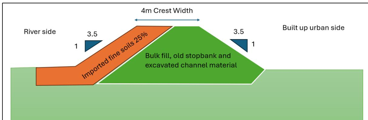
Figure 7.1: Adopted stopbank geometry (not to scale)
